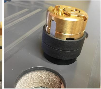
3. Apply two strips of sealing with spacer fitted.
