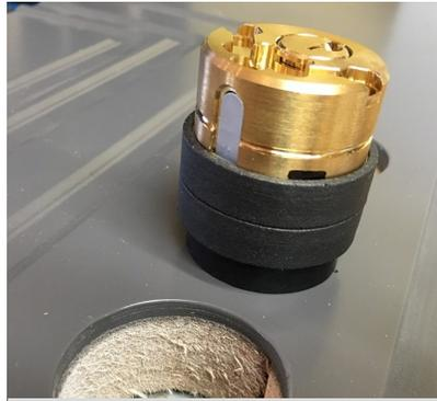
3. Apply two strips of sealing with spacer fitted.
